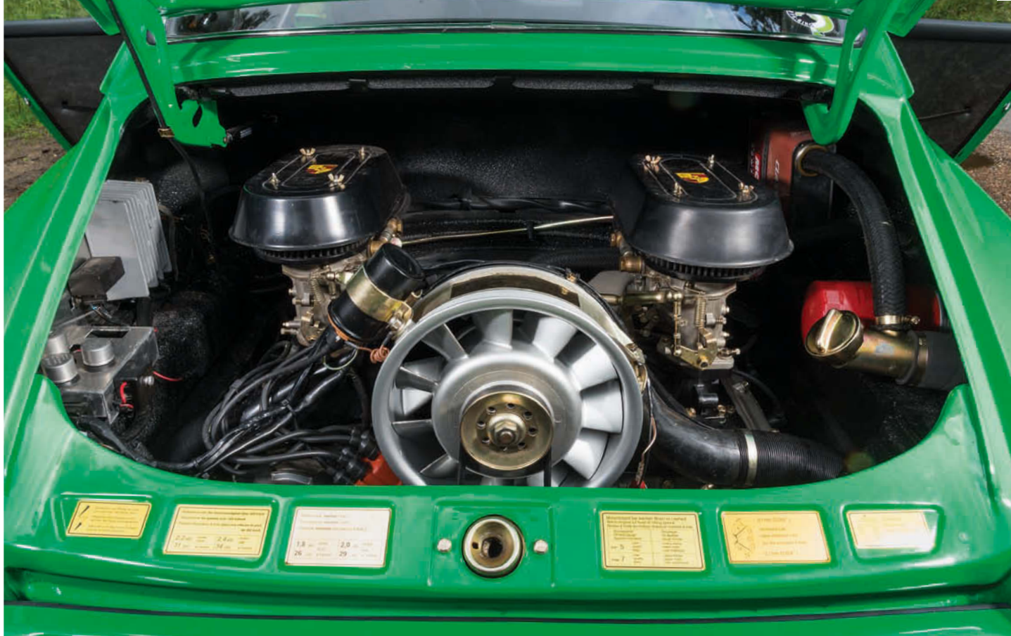
The engine's capacity has been raised from 2.2- to 2.4-litres, designed to make it handy in the Italian Alps
